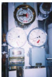
Below this photo are the controls for flooding 'B' magazine, located in 'A' magazine to the left of the door to 'B' magazine. The large wheel is for activating sprinklers, whilst the smaller wheel is for rapid flooding.
